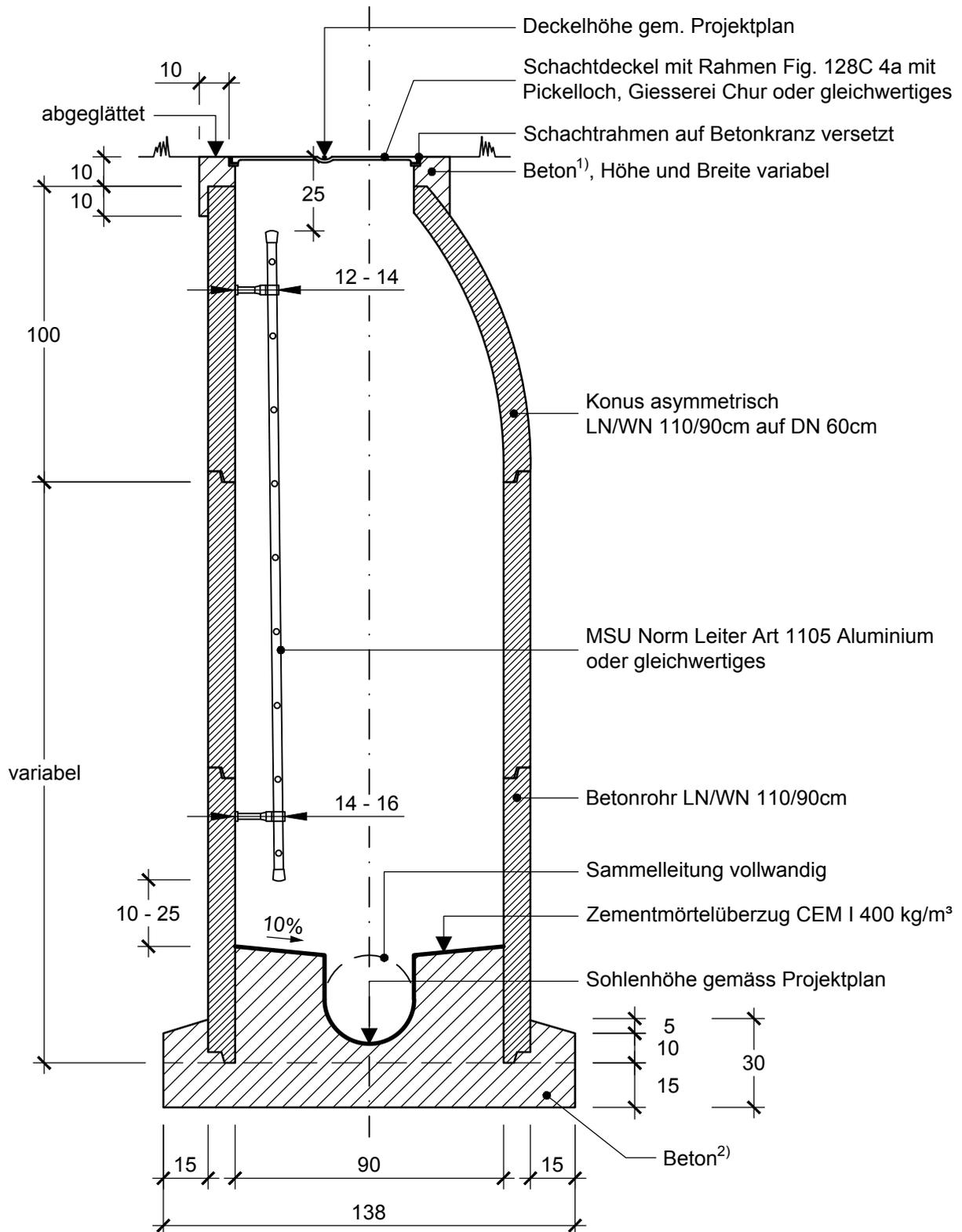
1) Beton: C 25/30, XF2 (CH), Dmax 16, CI 0.10 (SN EN 206-1)
